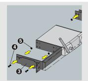
Use the fixing screws (4) and nuts (5) to screw the short brackets (3) on both Ubrackets. The short brackets, fixing screws and nuts are contained in the supplied rack mounting kit.
