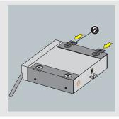
Insert one connecting strip (2) into each free slot in the side panel of the first receiver, making sure to align the hole in each connecting strip with the appropriate threaded hole in the receiver bottom panel.
