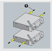
Unscrew the two fixing screws (1) from the right-hand side panel of one receiver and from the lefthand side panel of the other
