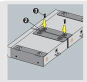
To join the two receivers, slide the connecting strips (2) on the first receiver through the free slots in the side panel of the second receiver. Make sure to align the hole in each connecting strip with the appropriate threaded hole in the bottom panel of the second receiver. Fix the connecting strips on the second receiver using the screws (3) from the supplied rack mounting kit.
