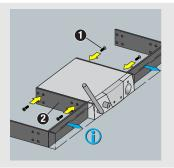
Use the fixing screws (1) to screw two U-brackets (2) on the receiver. The U-brackets are contained in the supplied rack mounting kit,
