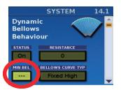
This parameter has no effect with the "Fixed Low," "Fixed Med," or "Fixed High" bellows curves.
