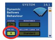
This "MIN BEL" parameter allows you to choose a minimum threshold for the bellows curve types. This parameter affects the "X-Light," "Light," "Standard," "Heavy," and "X-Heavy" settings.
